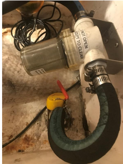
Sea Strainer and Thru Hull with Engine Key
