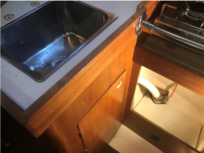
Galley Sink Thru-Hull Drain
