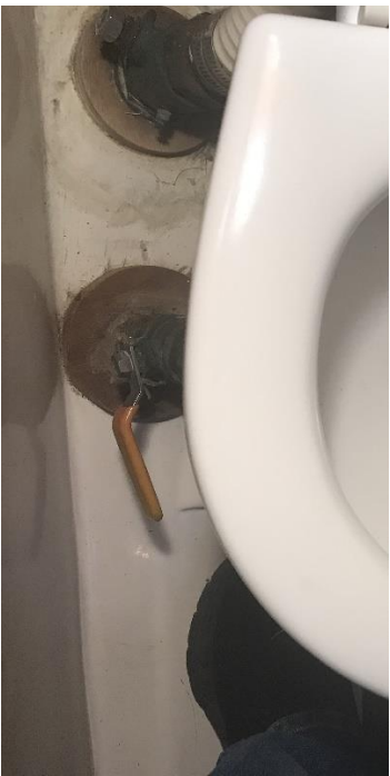
Head Thru Hull to Flush
