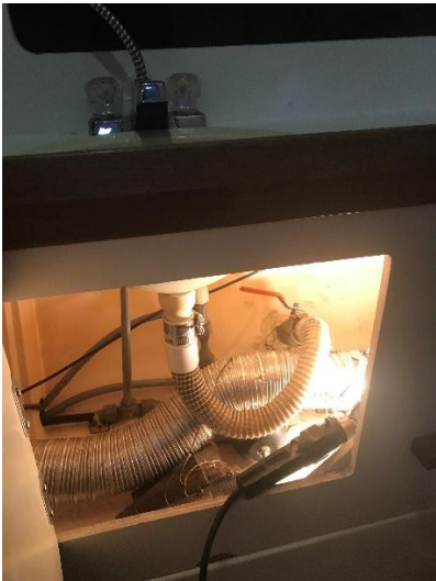
Head Galley Sink Thru-Hull Drain
