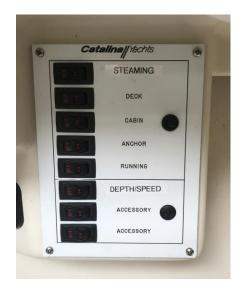
• The battery panel is on the starboard side inside the cabin. The switches operate fixtures as indicated on panel. MAKE SURE SWITCHES ARE SHUT OFF WHEN NOT IN USE.
